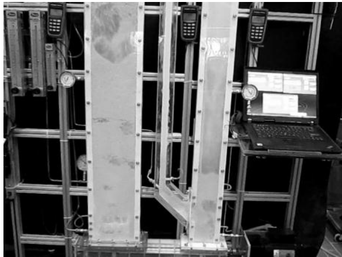
Figure 4.2: A picture of the cold unit system built at the Agricultural Research Service in USA, which is made from transparent Perspex sheets
