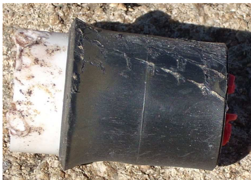
Figure 7.15: Deformation of part 3 and 4
