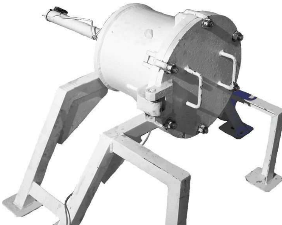
Figure 5.5: Purpose built stemming testing device with support legs.
