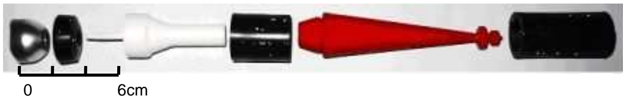
Figure 6.22: The mechanical plug disassembled.
