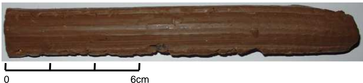
Figure 6.3: Photo of clay stemming capsule.
