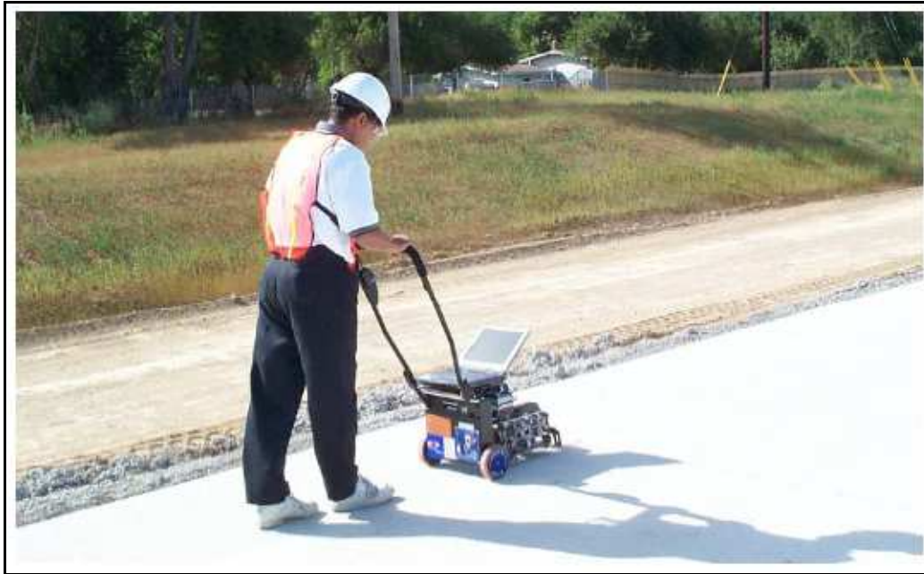
Figure 6: Walking Profilometer (Karamihas and Gillespie, 2002).
