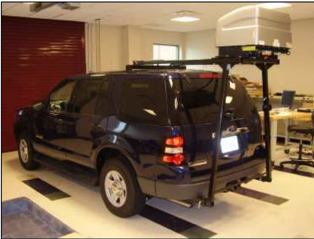
Figure 10: Vehicle Terrain Measurement System mounted on host vehicle (Kern, 2007).
