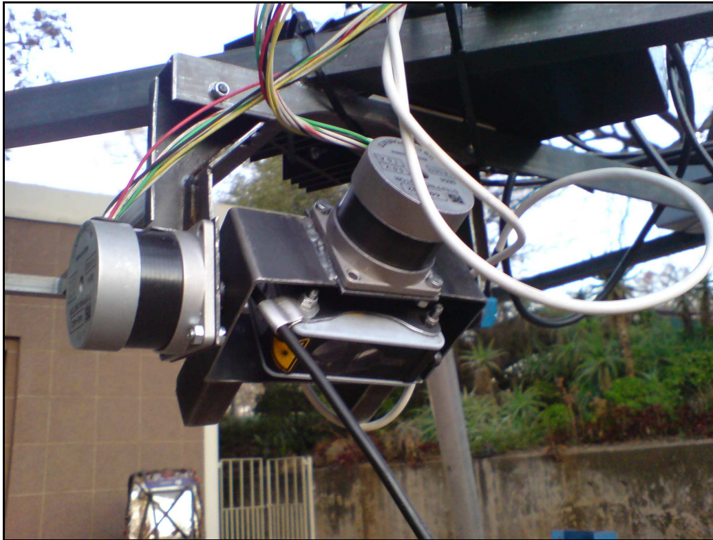
Figure 50: Gimball containing two stepper motors and a DM-80 Laser Distance Sensor.
