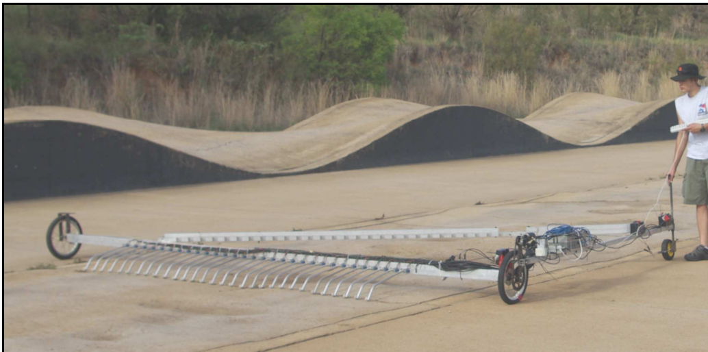
Figure 20: The Can-Can Machine on the Fatigue track at Gerotek.
