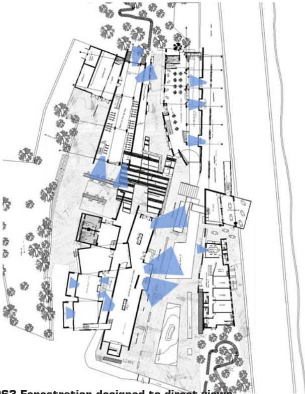
Fig. 063 Fenestration designed to direct views
