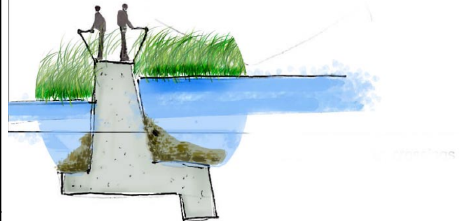
FIGURE 89 - Weir of filtration pond acting as pedestrian bridge, Author, 2008
