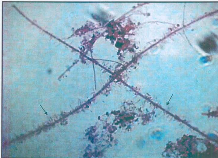
Fig. 7. Gram positive filament with attached epiphytic growth, Type 0041 (1000x) from Centurion WWTP foaming activated sludge.
