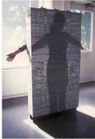
Illus. 125 (left) Litracon, Light Transmitting Concrete. (LITRACON 2007)
