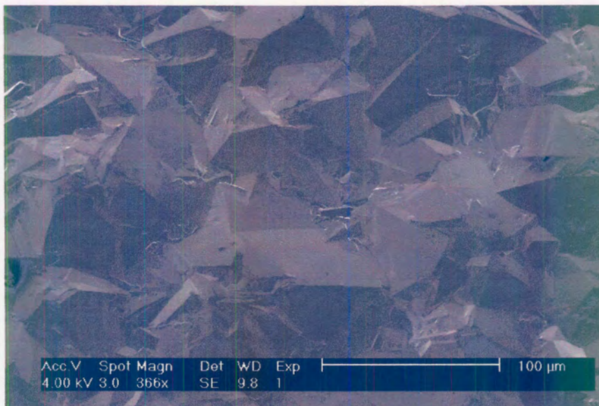
Figure 5.8 : SEM image of the as-received CVDBD4(2) sample
