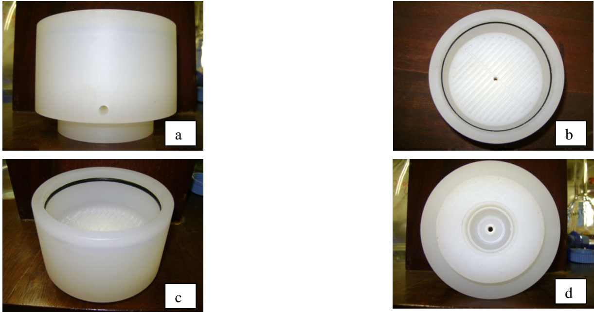
Fig. 3.2: a) Side view of column base showing opening to which vacuum was connected, b) Top view of column base showing grooved ‘floor’, drainage outlet and imbedded O-ring, c) Side view of column base showing the imbedded O-ring to ensure a vacuum tight seal between column and base, d) Bottom view of column base showing drainage outlet and threaded opening to which a Schott Duran glass bottle were screwed/fitted.
