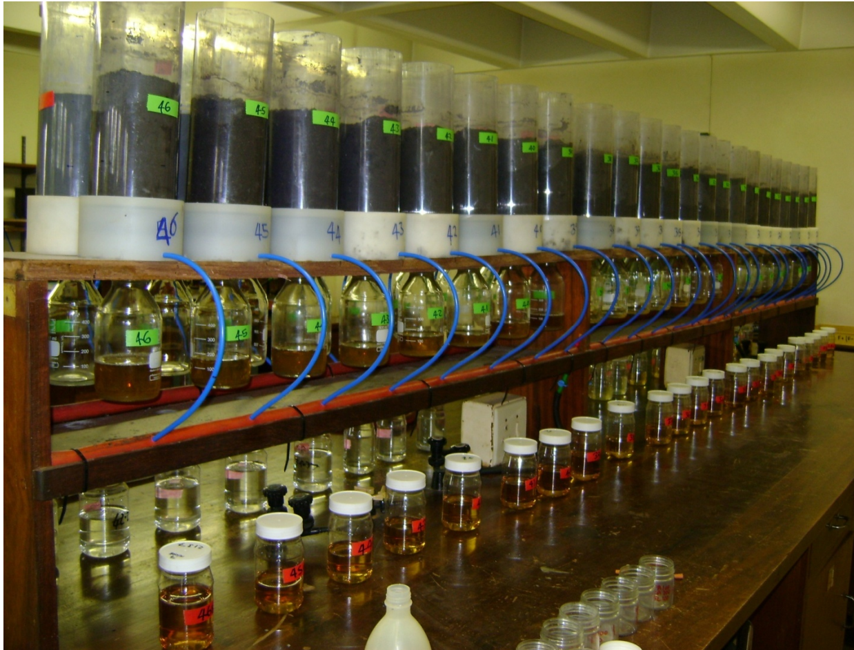
Fig. 3.4: The low tension column battery on each bench, connected to the vacuum system (blue pipe from column connected to the red main vacuum line) and collection plastic bottles.
