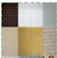
Carpets of synthetic fibres are more viable than natural fibres. Polypropylene fibre carpets will not shrink, are hostile to microbes and stains can easily be removed.
