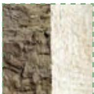
Different textural finishes can be achieved by dragging different objects over stucco plaster. By adding coarse river sand to plaster a coarser finish can be achieved, where stucco plaster floated with a wooden trowel can yield a finer texture.
