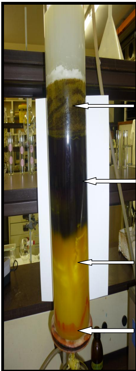
Figure 6. 6. Silica gel column chromatography of a methanolic extract of G. brighamii . The arrows indicate the separation of different phases of the extract with different solvent systems in the column.
