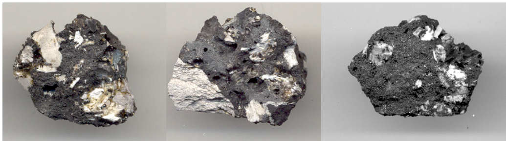
Figure 7.3: Hand-picked clinker fragments: “Stone” fragments (light colour) in black “glass” matrix.
