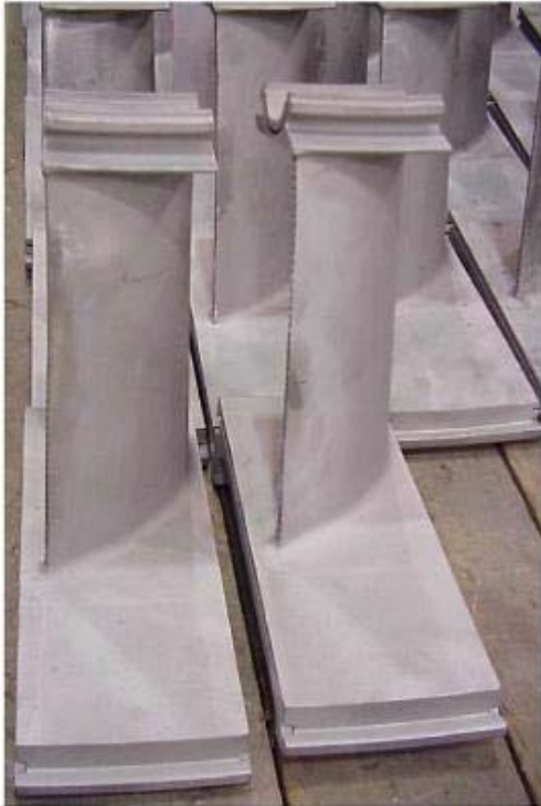
Figure 37 - V84.2 row 2 vane after complete repair including heat treatment and MCrAlY coating.
