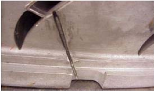
Figure 39(a) – Routed crack
