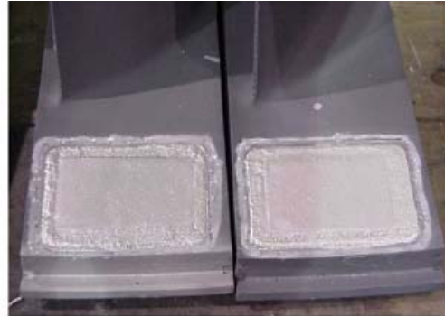
Figure 35 – V84.2, row 2 vanes repaired with the LPDB process.
