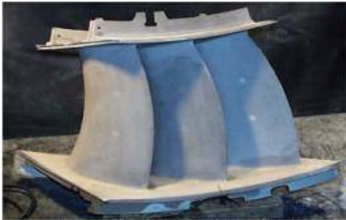
Figure 1 – View of W501F, Row 3 vane
