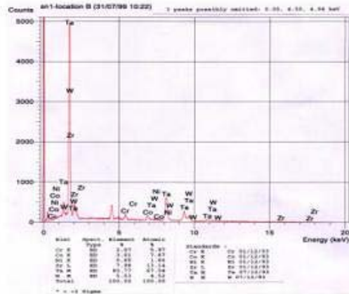
Figure 33 – Semi-qualitative and semi-quantitative analysis of the phase "B", along the grain boundary of a traditional type wide gap braze.
