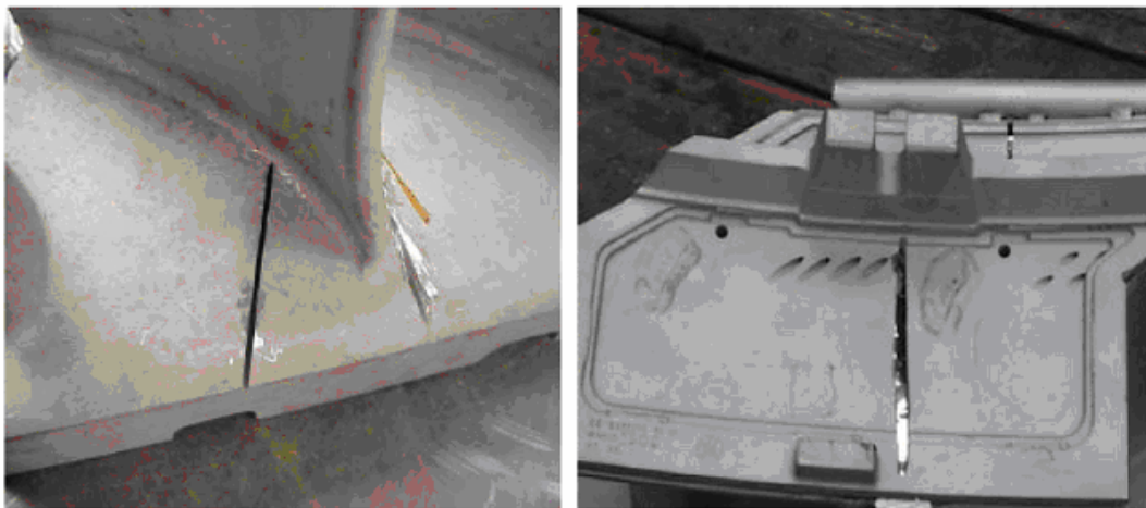
Figure 1: Ground out cracks on an X-45, W501F, Row 3 vane. Figure 2: Ground out cracks on an FSX-414, GE Frame 7EA vane.
