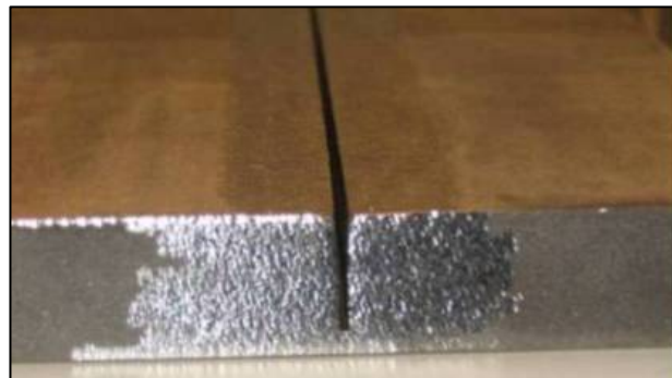
Figure 133 – Enlarged view of the 1.5 mm wide groove machined in the centre of the In738 plate samples.
