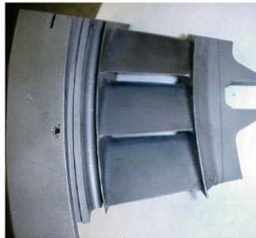
Figure 39 – Tornado, 2 nd stage stator segment after complete repair including heat treatment and Sermaloy J coating.
