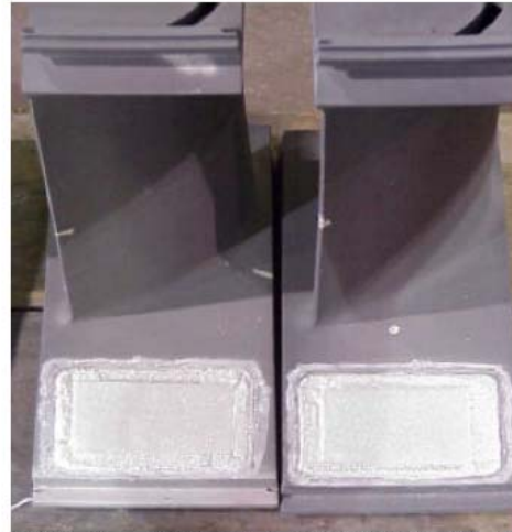
Figure 16 - V84.2, row 2 vanes repaired with the alternative wide gap braze process.
