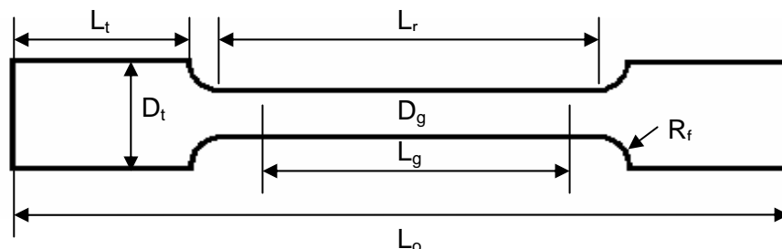
Figure 69 – Configuration of tensile and creep rupture specimens: D_g = 4.6 mm; L_g = 18.3 mm; L_r = 21.8 mm; L_o = 46.5 mm; R_f = 3.2 mm; L_t = 9.5 mm; and D_t = 8 mm.
