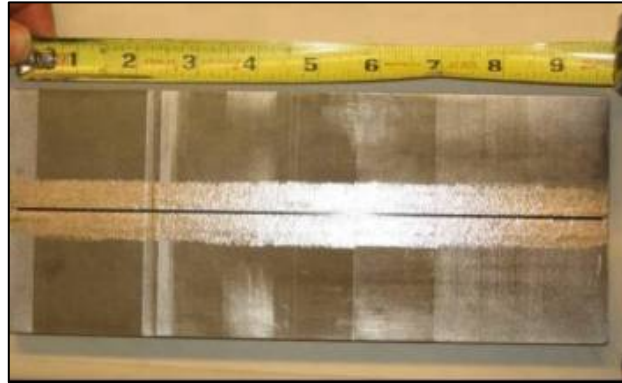
Figure 132 – In738 plate with a 1.5 mm wide groove machined in the center.
