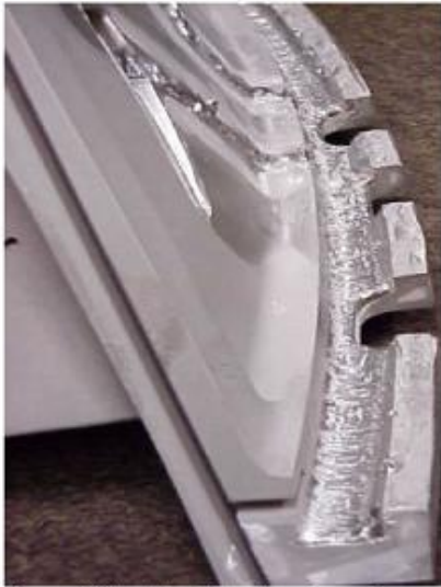
Figure 42(a) – Hook fit restoration, using paste.
