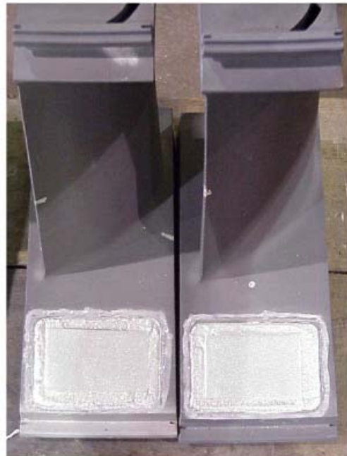
Figure 36 – V84.2, row 2 vanes repaired with the LPDB process.
