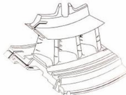
Figure 2 – Typical view from the concave side, showing leading edge, trailing edge and shroud/buttress cracking on the Alstom Tornado 2nd stage stator segment.
