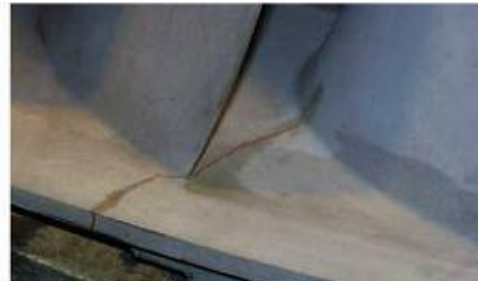
Figure 3 – Typical crack on the vane segment
