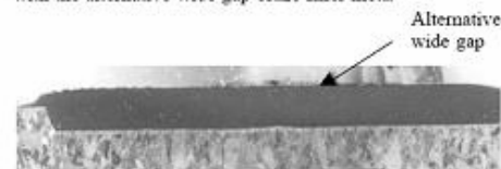
Figure 7 – Macrograph taken through the alternative wide gap braze repaired area of the V84.2, row 2 vane. Mag. 5X
