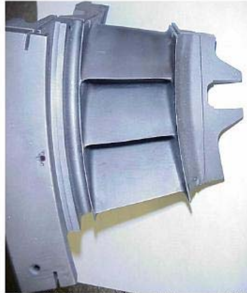
Figure 38 – Tornado, 2 nd stage stator segment after complete repair including heat treatment and Sermaloy J coating.
