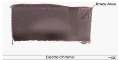
Figure 43 – Macrograph taken through a crack repaired with the "Sermafill" process
