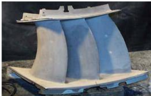
Figure 1 – View of W501F, Row 3 vane
