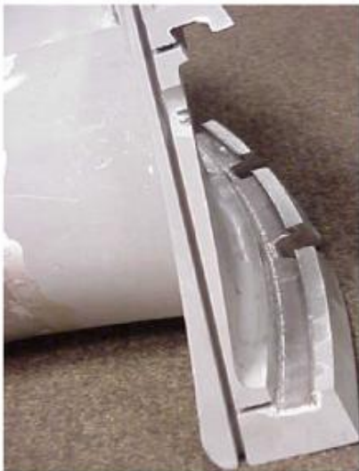
Figure 42(b) – Hook fit restoration, using pre-sintered plate.
