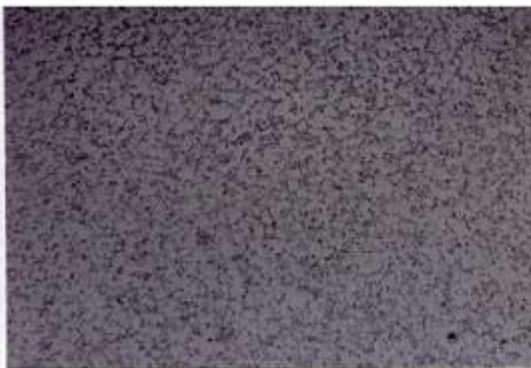
Figure 11 – LPD Bonded “Sermafill’ed joint on a X-45 substrate. Mag.100X
