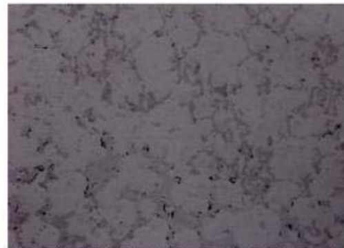
Figure 13 – LPD Bonded “Sermafill’ed” joint on a X-45 substrate. Mag. 500X
