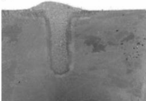
Figure 10 – Macrograph of the joint taken through the alternative wide gap braze repair of the Tornado, 2 nd stage stator segment. Mag. 5X
