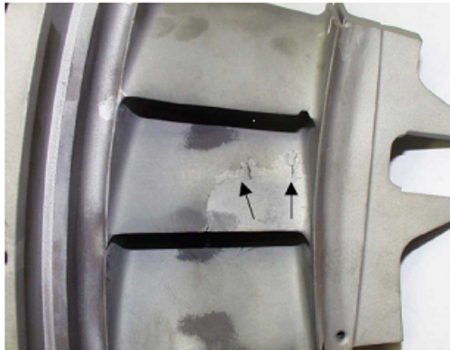
Figure 11 – Strain age cracking, on the airfoil, after initial attempts at a weld repair.
