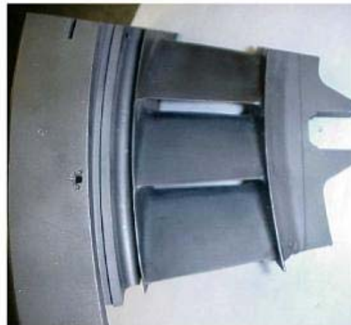
Figure 39 – Tornado, 2 nd stage stator segment after complete repair including heat treatment and Sermaloy J coating.
