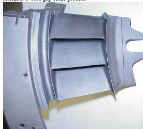
Figure 17 - Tornado, 2 nd stage stator segment after complete repair including heat treatment and Sermaloy J coating.
