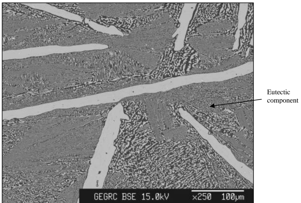
Figure 142 - BSE image of the Ni-13Cr-25 Hf alloy showing primary \text{Ni}_7\text{Hf}_2 , and a fine eutectic component consisting of \gamma phase and the \text{Ni}_7\text{Hf}_2 intermetallic compound.
