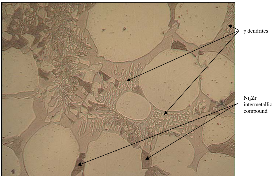
Figure 80 - Ni-Zr braze dispersed between MarM247 powder particles after brazing at 1230°C for 40 minutes. Magnification: 500X.
