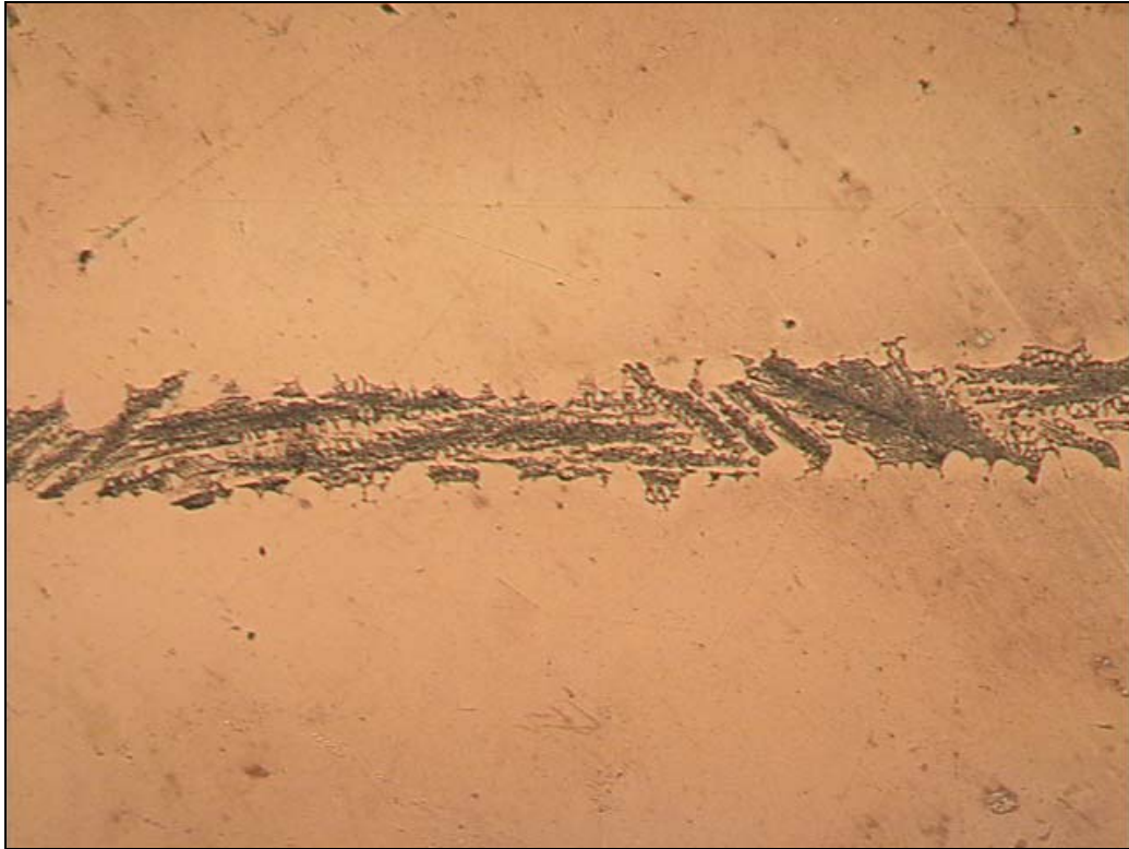
Figure 60 – Optical micrograph of a Ni-Hf brazed joint in In738 parent metal after brazing at 1230°C for 18 hours. Magnification: 100X.
