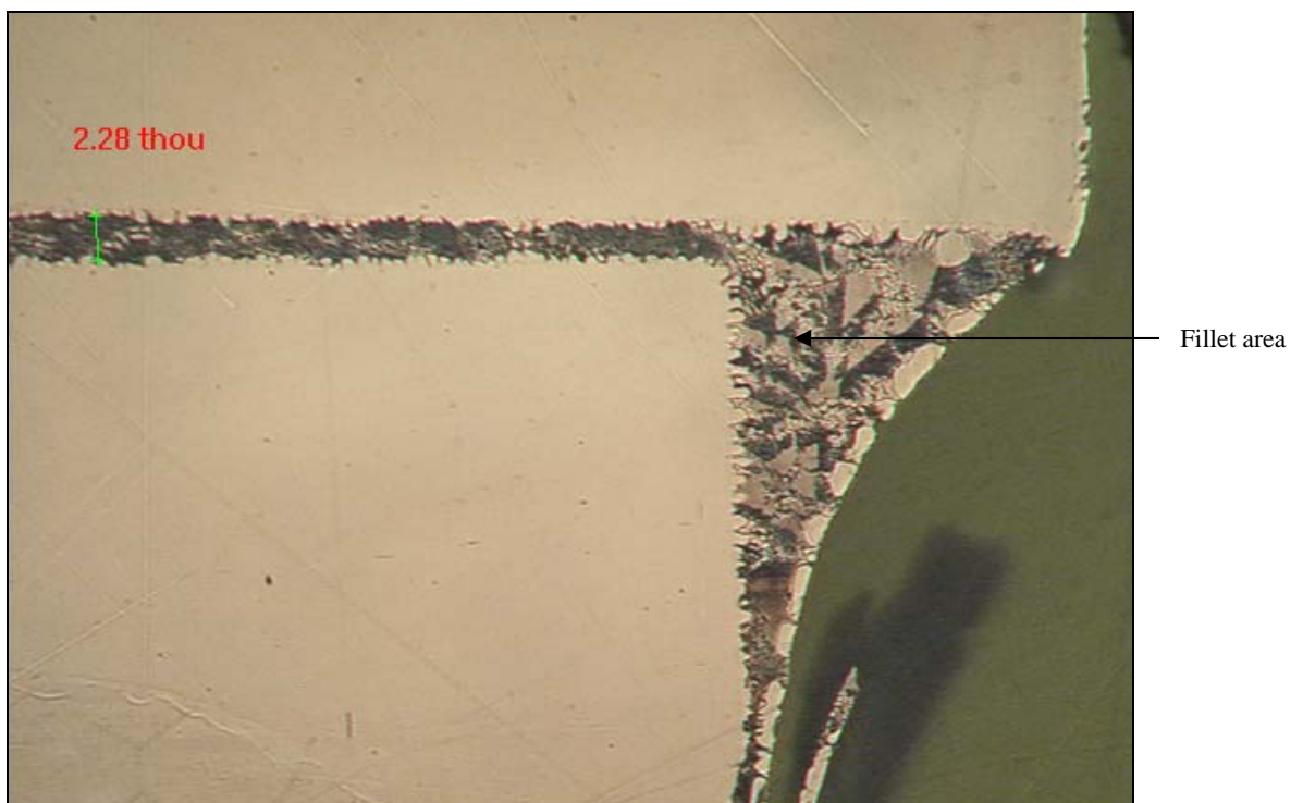
Figure 54 – Optical micrograph of a Ni-Zr brazed joint in In738 parent metal after brazing at 1230°C for 40 minutes. Magnification: 50X.
