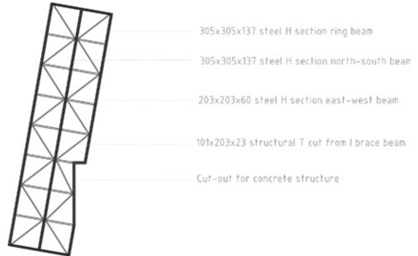
Fig 9.9: Plan of steel floor frame
