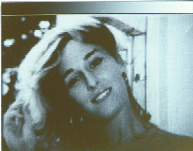
Figure 13 GIRL coded using a DCT of size 4x4, 1.0 bits/pel.
