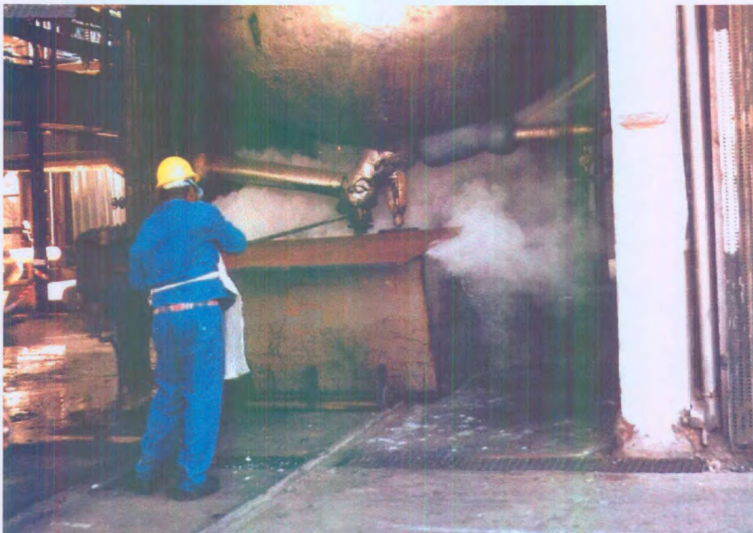
Figure 2.4 Draining of phthalic anhydride residue from a main distillation kettle.
