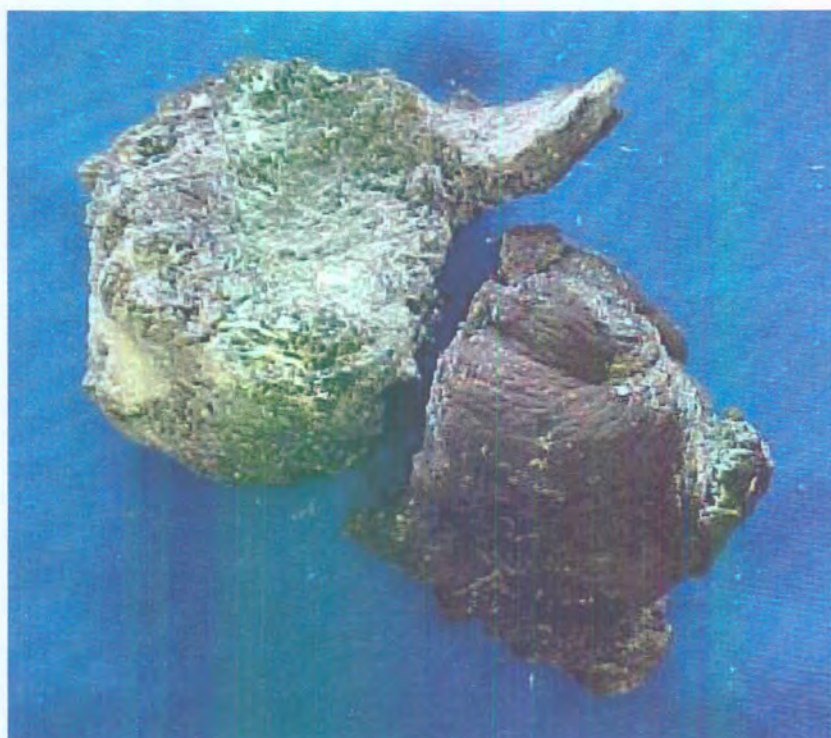
Figure 4.6 Final phthalic anhydride residue after treatment with Dicalite 4151 (Experiment F).
