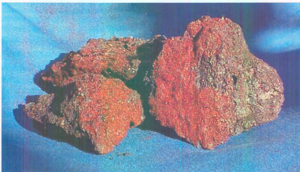
Figure 4.1 Sample of phthalic anhydride residue after distillation.
