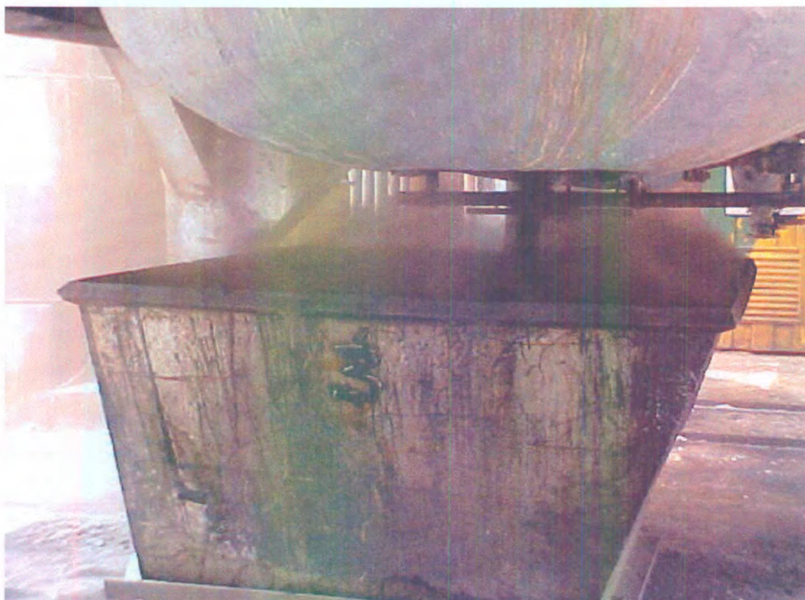
Figure 4.10 Residue mixture released into a disposal trolley after distillation and treatment with Dicalite 4151 (Experiment I).
