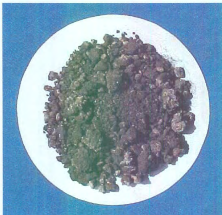
Figure 4.7 Final phthalic anhydride residue after treatment with Dicalite 4151 (Experiment G).
