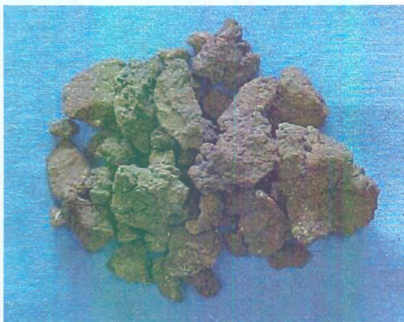
Figure 4.5 Final phthalic anhydride residue after treatment with Dicalite 4151 (Experiment E).
