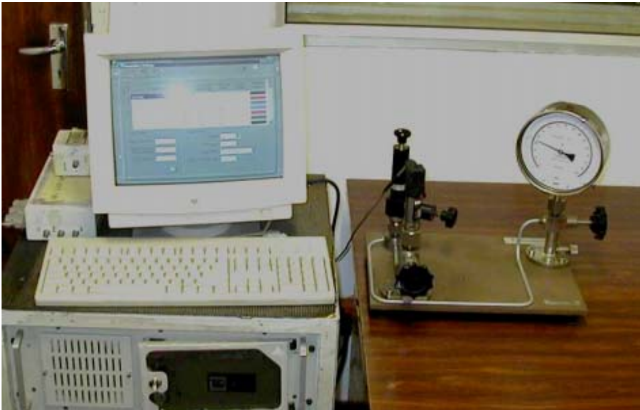
Figure C.1 Pressure Transducer Calibration Layout.
