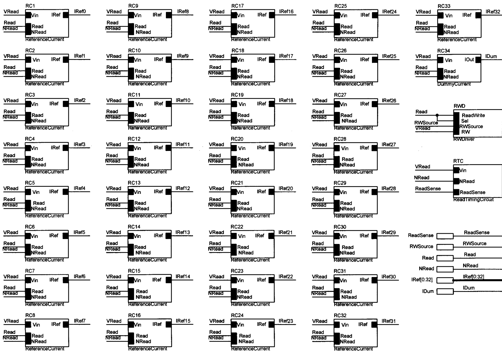
Figure C.29 Reference Circuit: Array of reference current generators with driving circuit.
