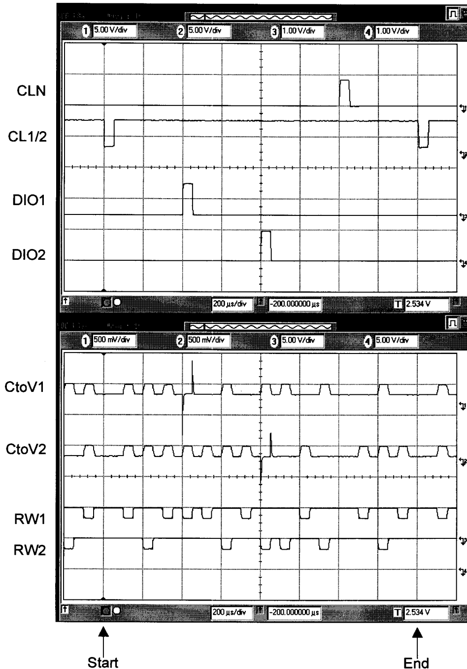
Figure 2.28 Experimental results for the sequence that tests clearing the cell via the NMOS source.
