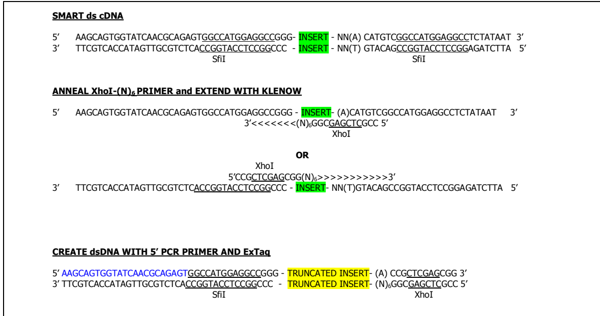
Figure 4.7. Schematic representation of fragmenting the full-length SfiI library using random primers.
