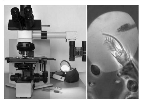
**Fig. 9** Apparatus for drawing fine details: inverted binocular placed under the drawing tube opening (on the *left*) to decrease the size of the pencil or pen relative to small structures, such as empodia (on the *right*)
