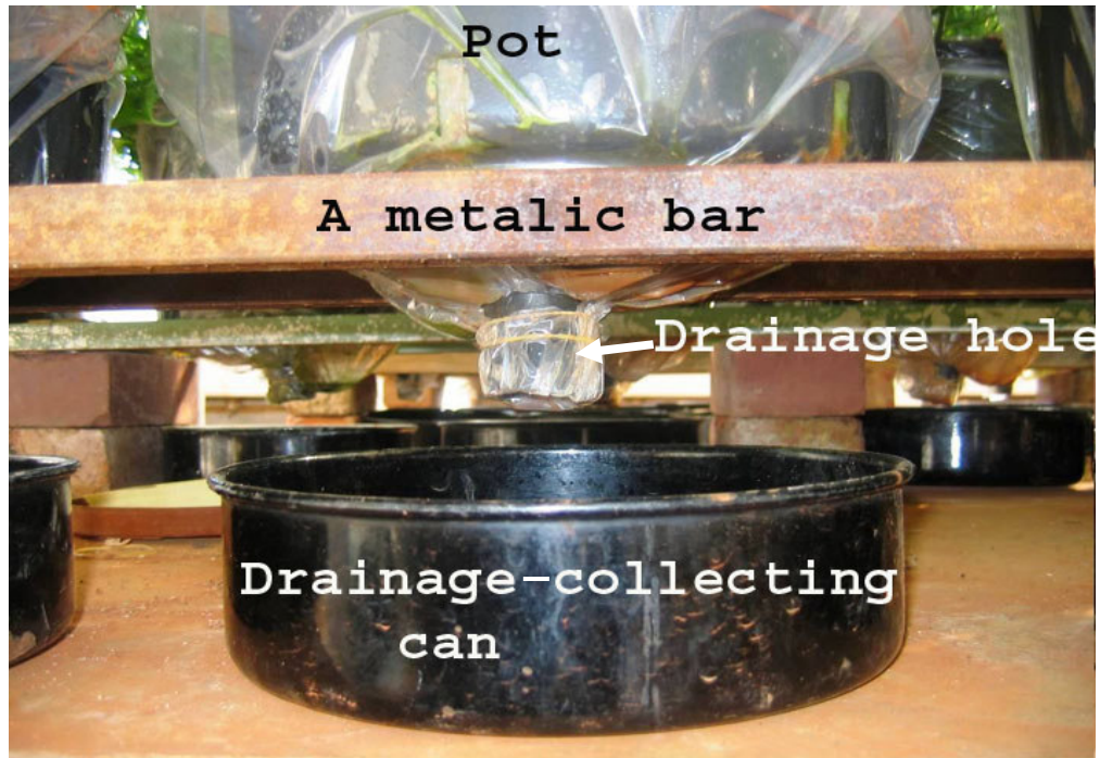
Figure 5.2: Drainage-collecting container in the glasshouse pot trials
