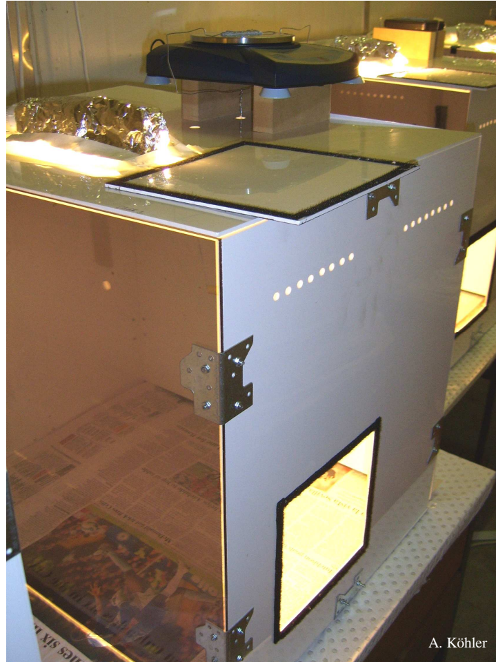
Fig. 2. The Perspex cages used for the fasting experiment in brown honeyeaters (Chapter 3). One side of each cage consisted of a one-way mirror allowing for observation of the bird with minimal disturbance. The only perch available in the cage was suspended from a balance which was placed on top of the cage. Body mass was recorded manually when the bird was resting on the perch. The feeder was attached outside the cage, allowing for weighing of the feeder without disturbance of the bird.
