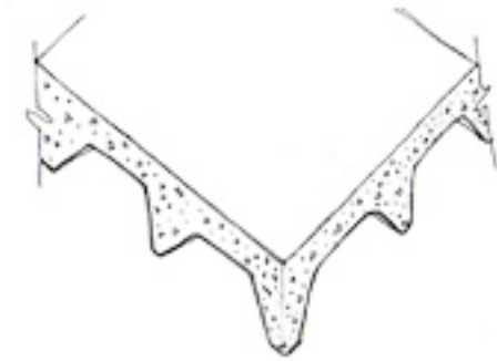
Typical coffered slab 3d extract
