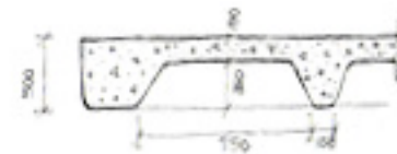
Typical coffered slab profile
