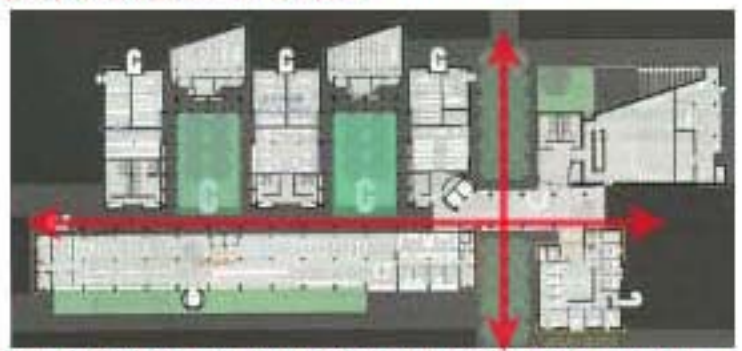
Tuks law building designed around two central courtyards that act as communal space. The courts are also placed adjacent to the circulation space.
