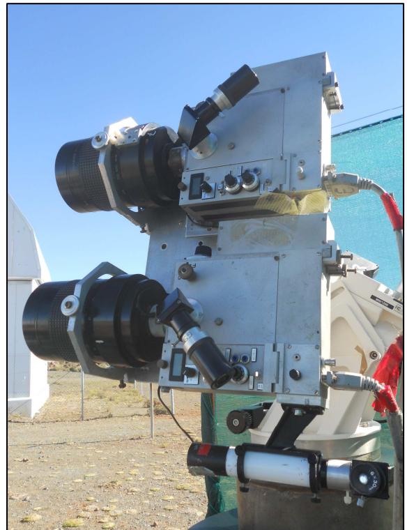
Figure A4.3. The GSM at Sutherland operated in DIMM mode with the two Maksutov telescopes sharing the same mount.
