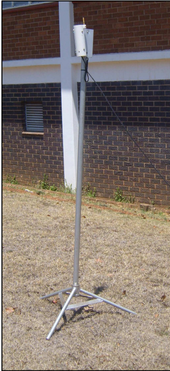
Figure A4.6. The Boltwood Cloud Sensor at HartRAO.
