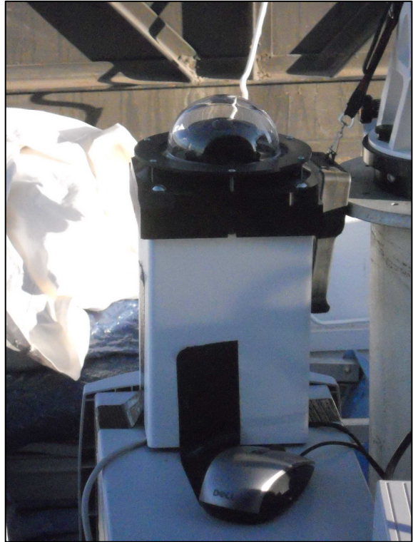
Figure A4.7. The SAAO All Sky Camera at Sutherland is located together with the SALT MASS-DIMM in the ox wagon enclosure.
