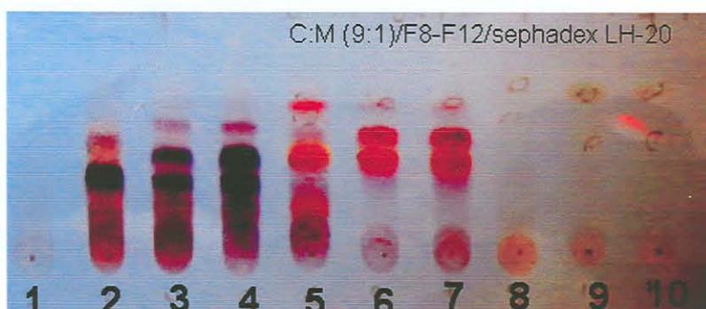
Figure 5-13: Chromatogram of the separation of 2.5 g of F 2 -F 12 combined fraction on Sephadex LH-20 separated with chloroform/methanol (9:1) solvent system and sprayed with vanillin sulphuric acid spray reagent.
