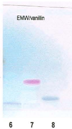
Figure 5-17: Chromatogram (developed in EMW sprayed with vanillin sulphuric acid spray reagent) of compounds isolated from C. padoides .
