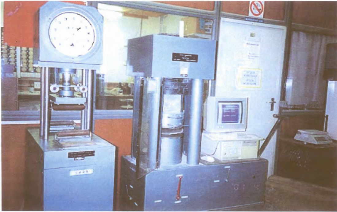
Photo G.7: Determining compressive strength of concrete in cube press
