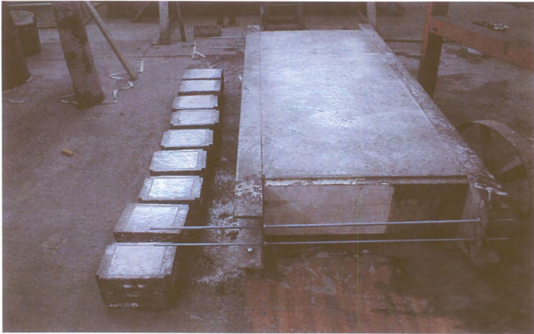
Photo G.3: Beam and air-cured cubes
