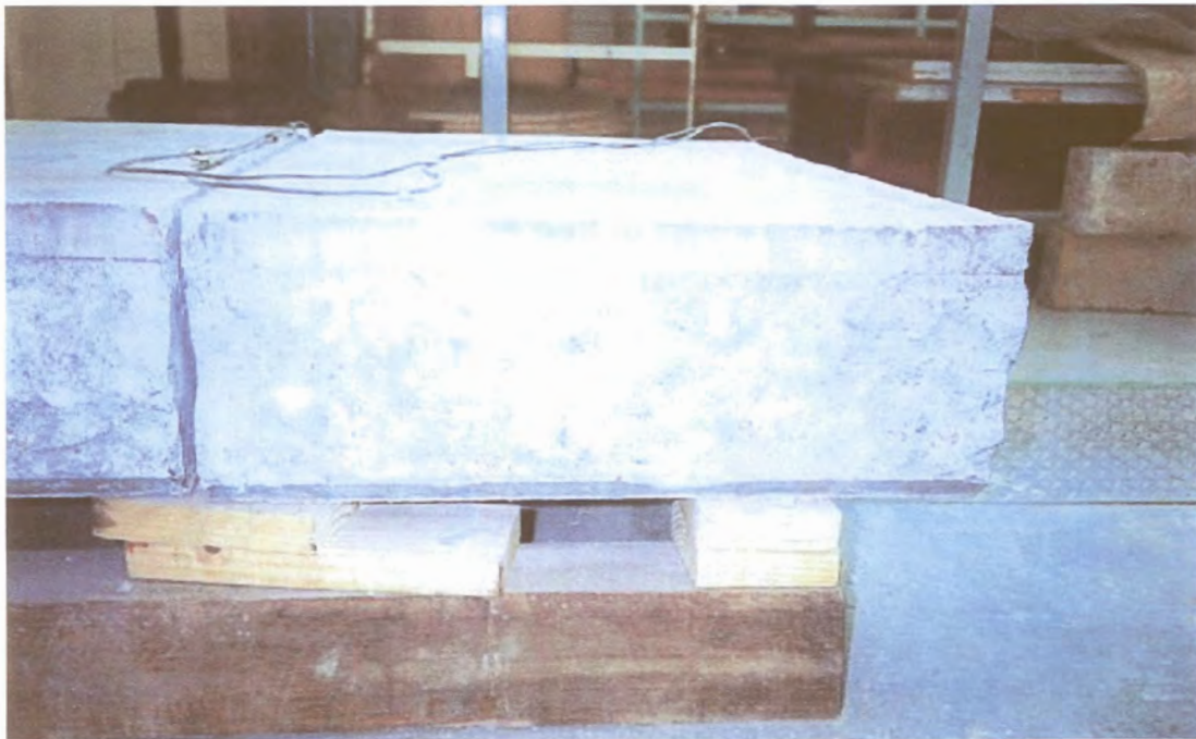
Photo G.20: Crack face of 37,5 mm granite aggregate test beam – Experiment 2
