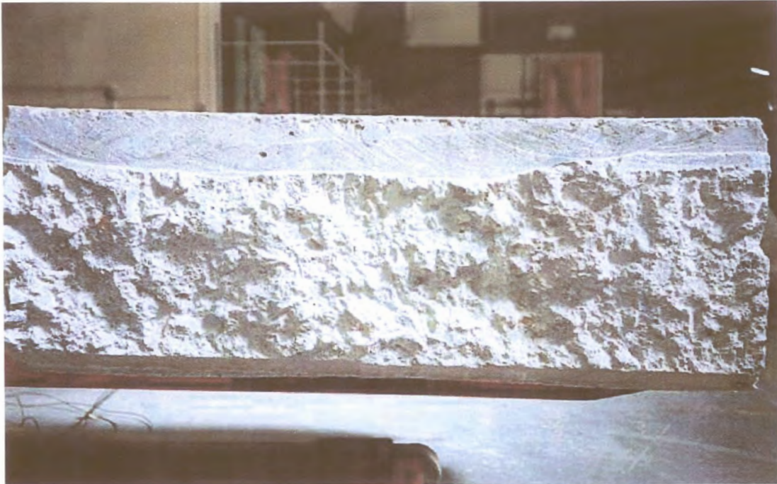
Photo G.19: Crack face of 19 mm granite aggregate test beam – Experiment 1
