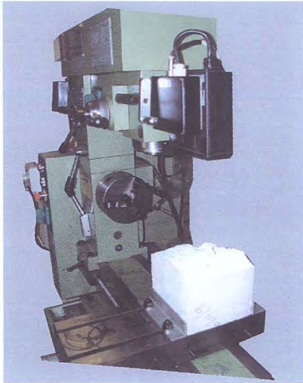
Photo G.25: Laser measuring unit mounted on a milling machine to obtain Volumetric Surface Texture (VST) measurement of concrete sample
