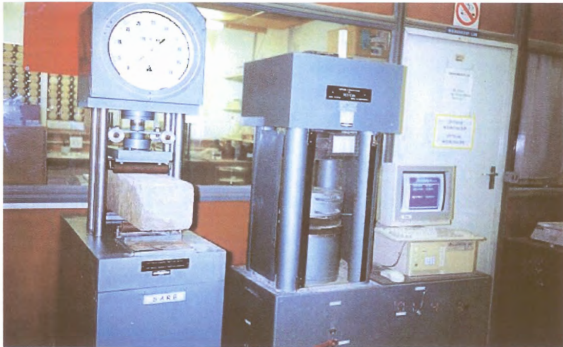
Photo G.8: Determining modulus of rupture of concrete in two-point loading press
