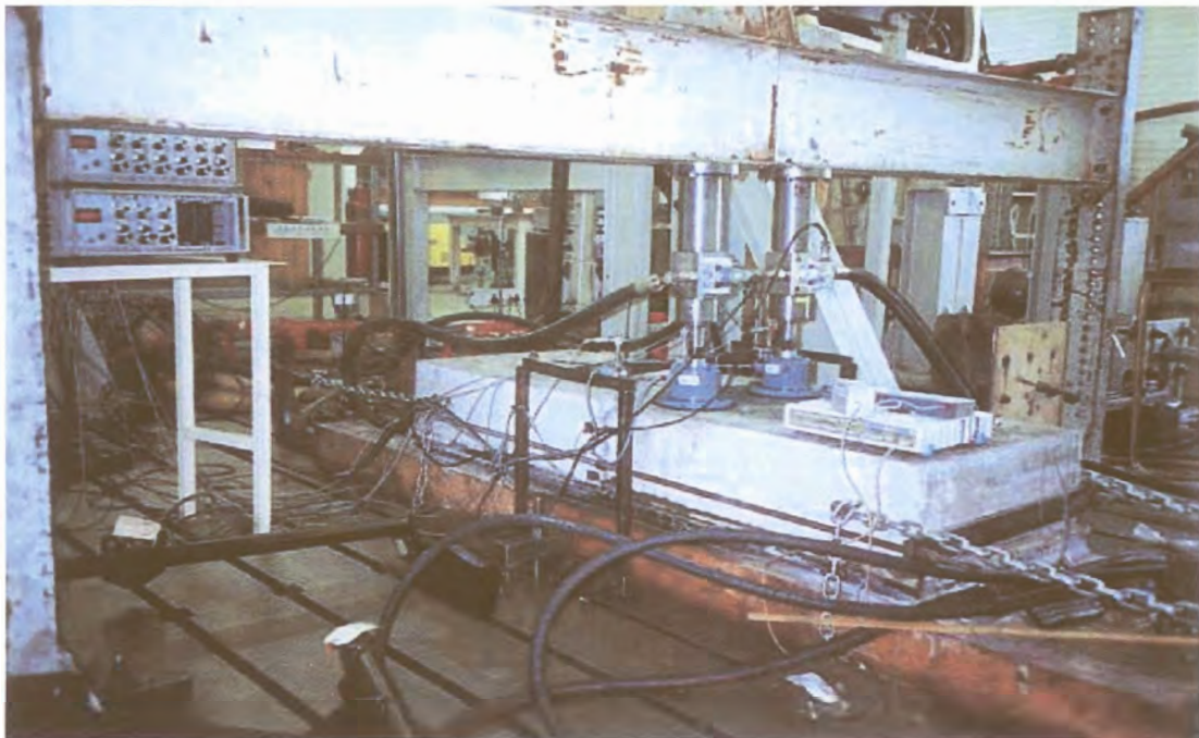
Photo G.16: 40 kN static loading with two actuators at one side of joint (Spider measuring temperature in beam in foreground) – Experiment 3
