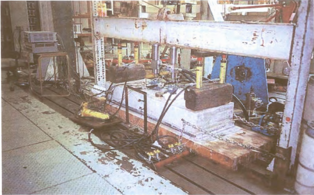
Photo G.15: Pressing down ends of beam to break crack open for testing at different crack widths – Experiment 3
