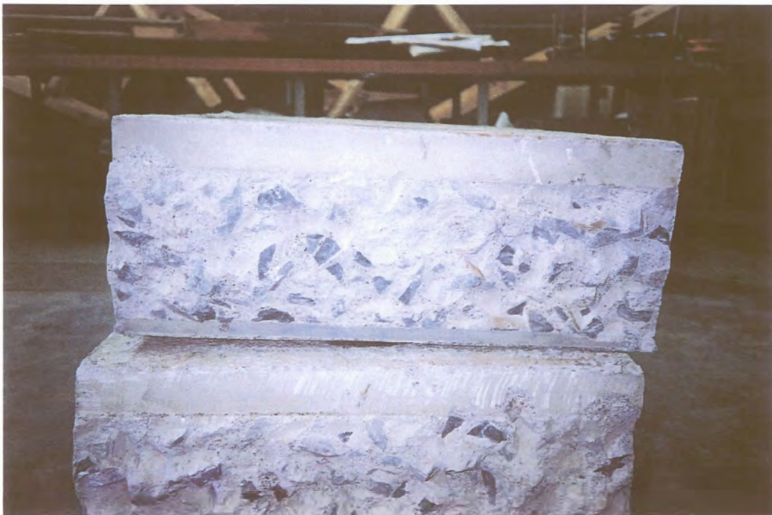
Photo G.22: Crack face of 37,5 mm dolomite aggregate test beam – Experiment 4
