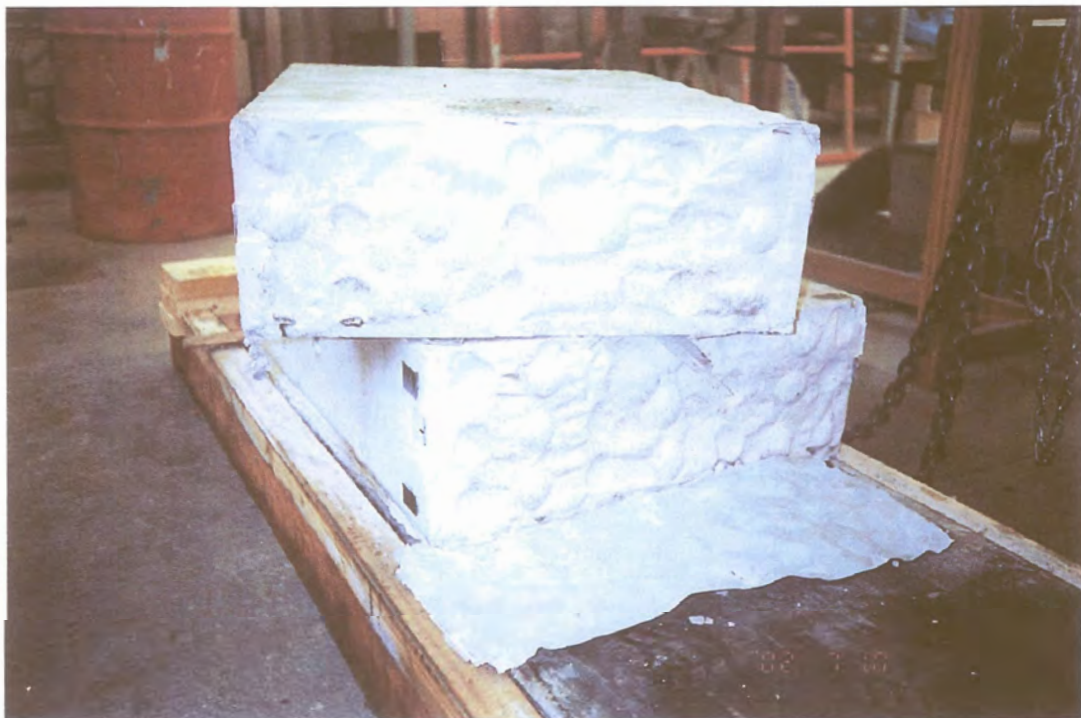
Photo G.24: Smooth face of pre-deformed plastic joint with plastic sheet in foreground – Experiment 5
