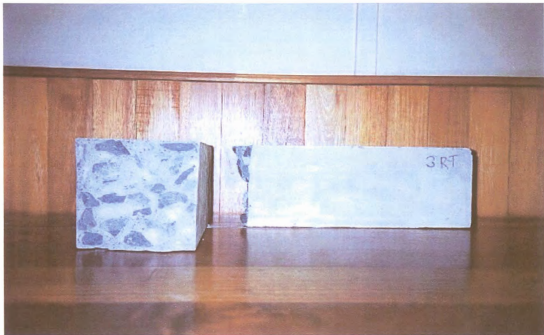
Photo G.10: Crack face of modulus of rupture test beam - 37,5 mm dolomite aggregate
