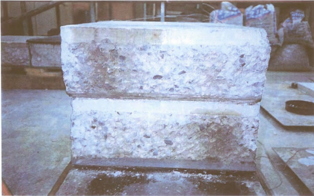
Photo G.21: Crack face of 19 mm dolomite aggregate test beam – Experiment 3
