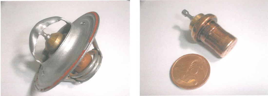
Figure 3.22 Thermostat and wax actuator
