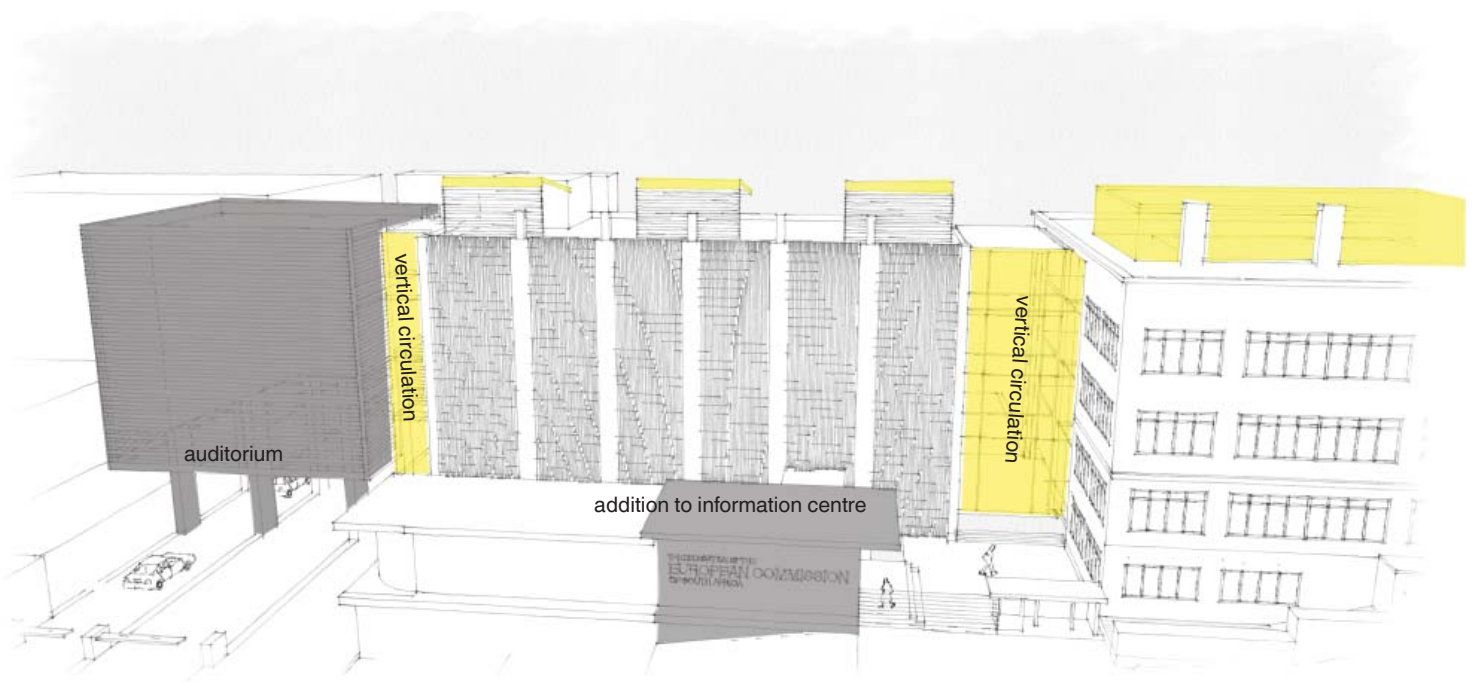
Fig.366: New and existing structure
