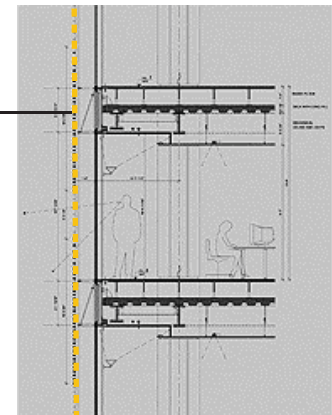
Fig.303: Section showing position of shading system [Source: http://www.arcspac.com/architects/pianoNYT/ ]
