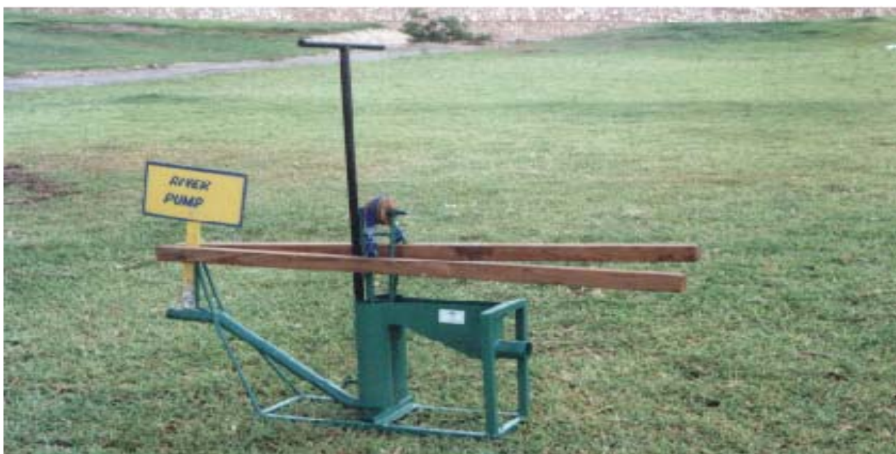
Figure 18: The river pump superstructure after installation.
