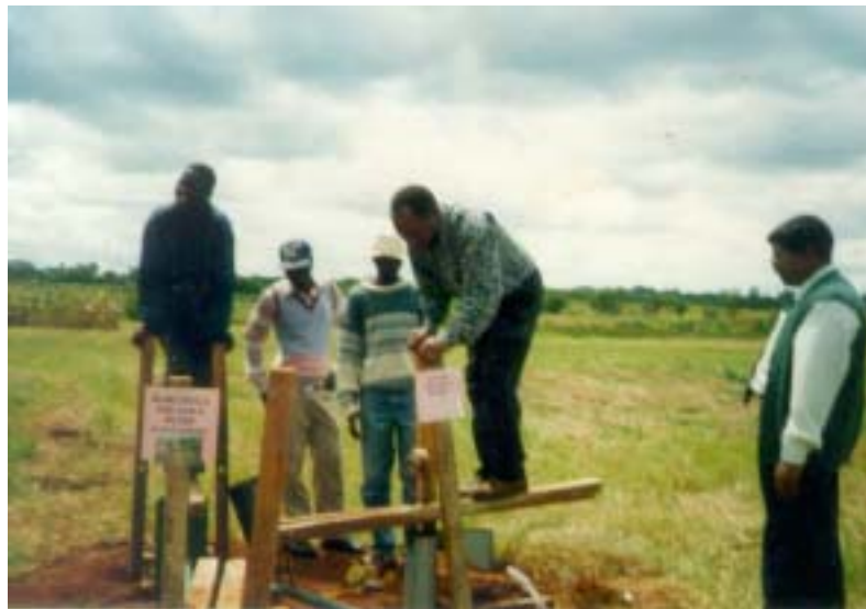
Figure 14: The Treadle pump in Operation Activated By Human Feet.
