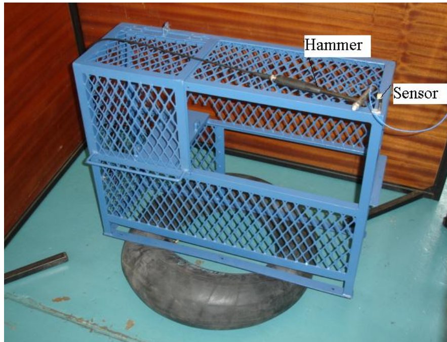
Figure 4.11 Modal analysis of frame structure
