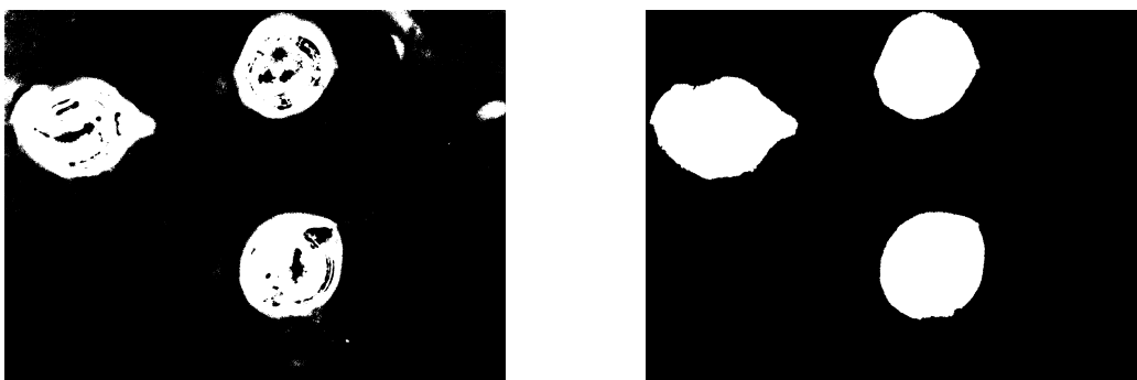
(a) Black and white image obtained after thresholding the grayscale image in figure B.1(b) (b) Cleaned black and white image ready for particle shape extraction
