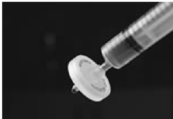
Fig 2.1 Whatman ® Puradisc polyethersulferone (PES) filter used for filtering the test solutions (with a syringe attachment)
