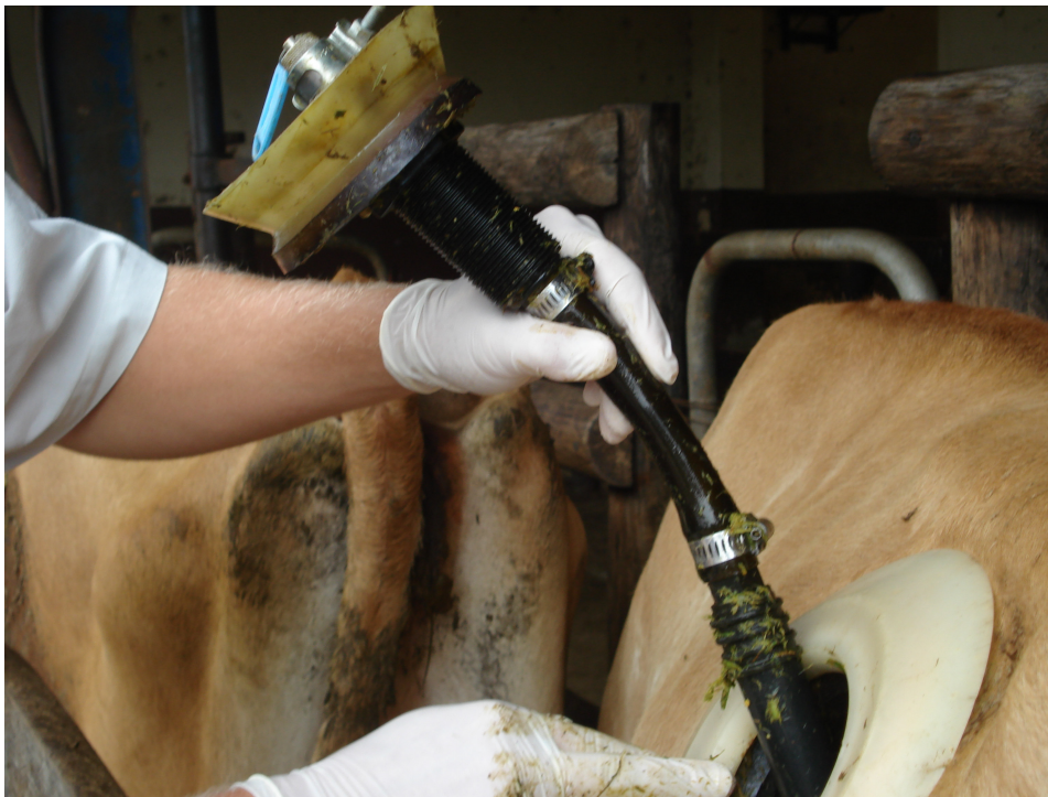
Figure 4.2: The new logging system being inserted through the cannula. Both the logger and the probe go into the rumen of the cow
