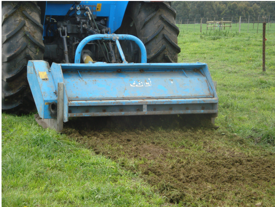
Figure 3.2: The mulcher used on the italian, westerwold and perennial ryegrass pasture treatments to create a seed-bed for the ryegrass seeds
