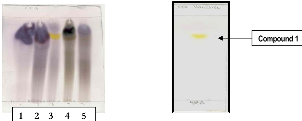
Figure 6.4: TLC profiles of pooled fractions from column chromatography of fraction 3 eluted with CEF. Sample from test tube 3 formed a pure Compound 1.
