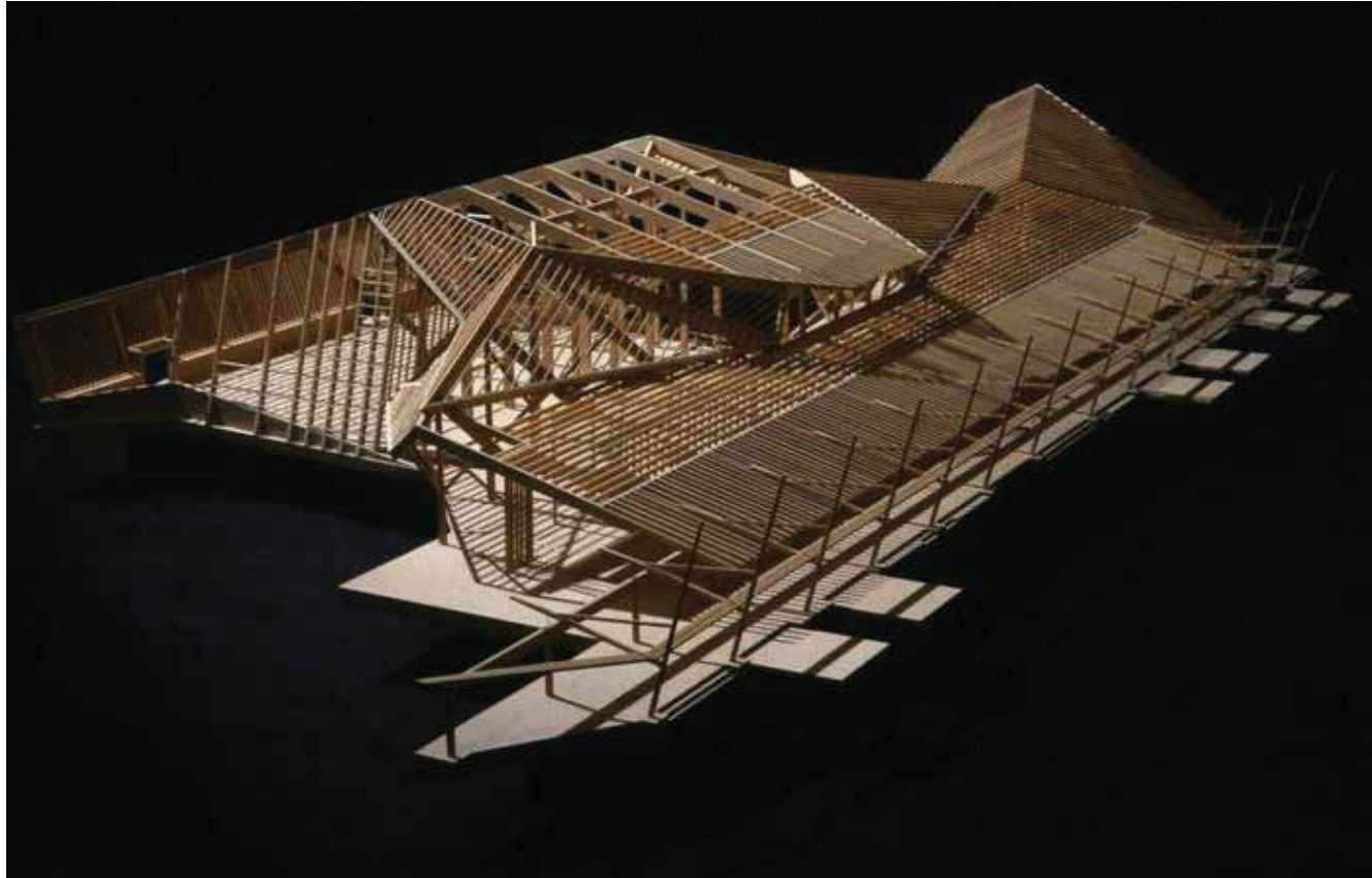
Figure - 6.5 (Above) - The heavily engineered structure was too complicated for the local builders to understand, so the architects built a exact physical model to explain the three dimensional characteristics of the tectonic roof structure. The model also depicts the changing nature of the roof structure and the different approaches to the opposite ends of the building.
