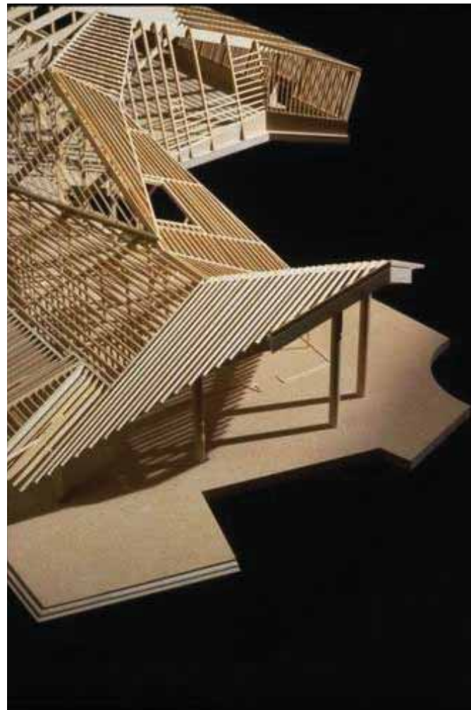
Figure - 6.5 (Above) - The heavily engineered structure was too complicated for the local builders to understand, so the architects built a exact physical model to explain the three dimensional characteristics of the tectonic roof structure. The model also depicts the changing nature of the roof structure and the different approaches to the opposite ends of the building.
