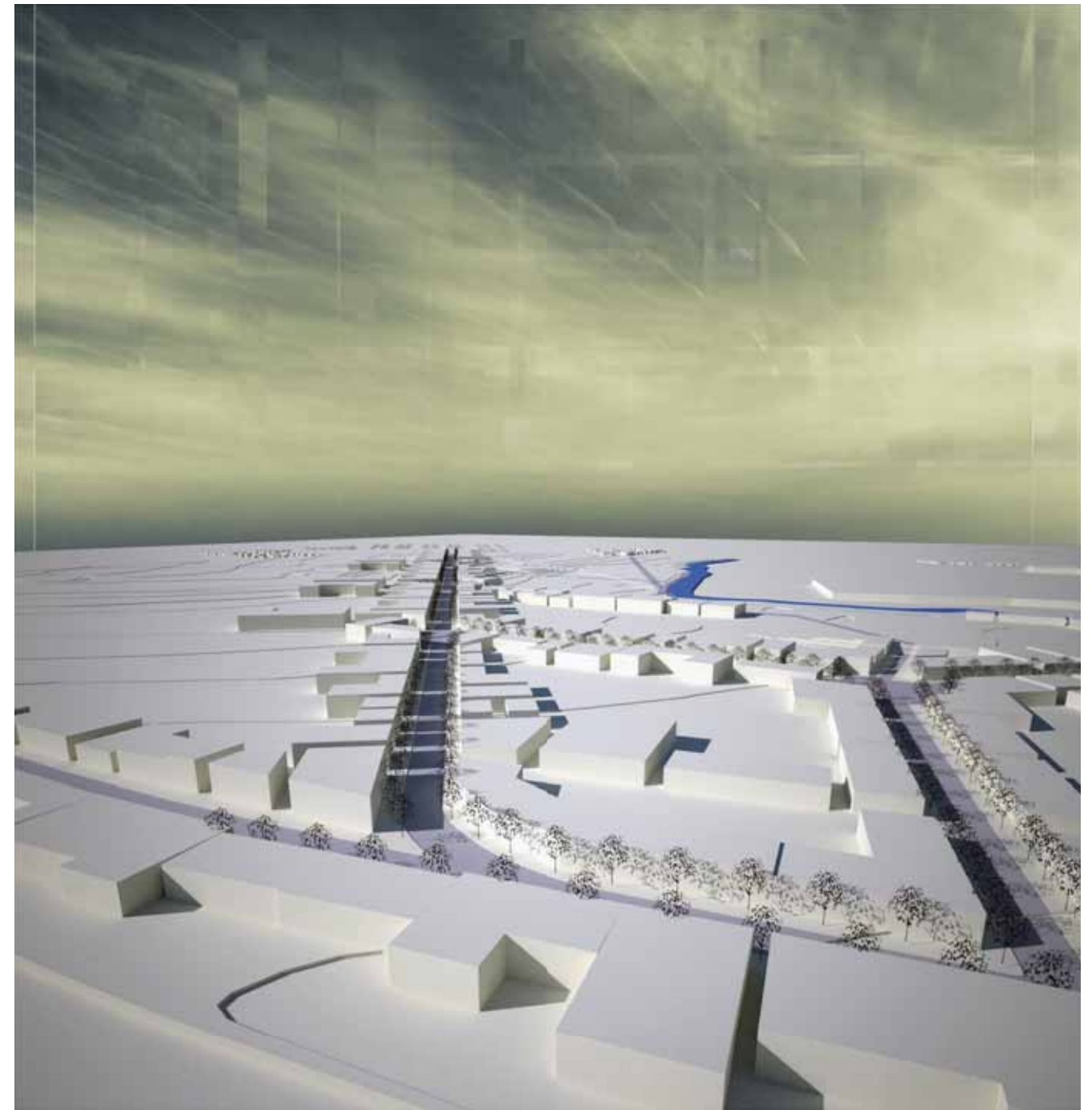
Figure - 5.32 - Rendered perspective view looking south down towards Nellmapius extension 3. This activity corridor acts as the connecting mechanism between the Eerste Fabrieke development and the residential area of Nellmapius. The left side of the corridor will be characterised by medium to high density housing and the right side by mixed use industry and medium density residential.
