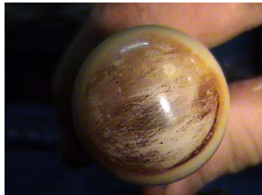
Figure 6.29 – The black deposit found on the femoral head of the station using a preserved steel post and bovine serum as test medium. The station completed 4 500 000 cycles.
