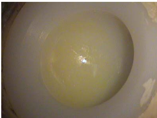
Figure 6.28 – A black deposit was found on the femoral head of the bovine serum station after 4 500 000 cycles. The station used an aluminium post.
