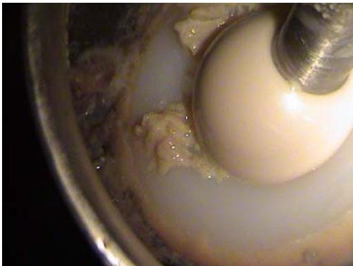
Figure 6.22 – The “seal” in station 4 after 4 000 000 cycles.
