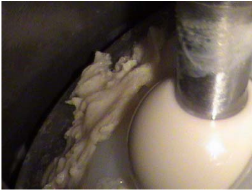
Figure 6.22 – The “seal” in station 4 after 4 000 000 cycles.
