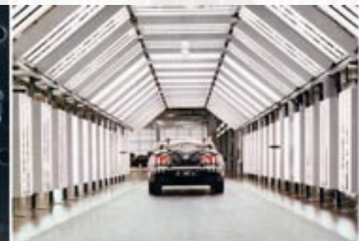
VW Phaetons gliding across a beauty queen promenade, a 25m long neon tunnel where the paint job is checked for blemishes. The finished cars are displayed in a glass arcade. [Champa, P. Surface, issue 43]
