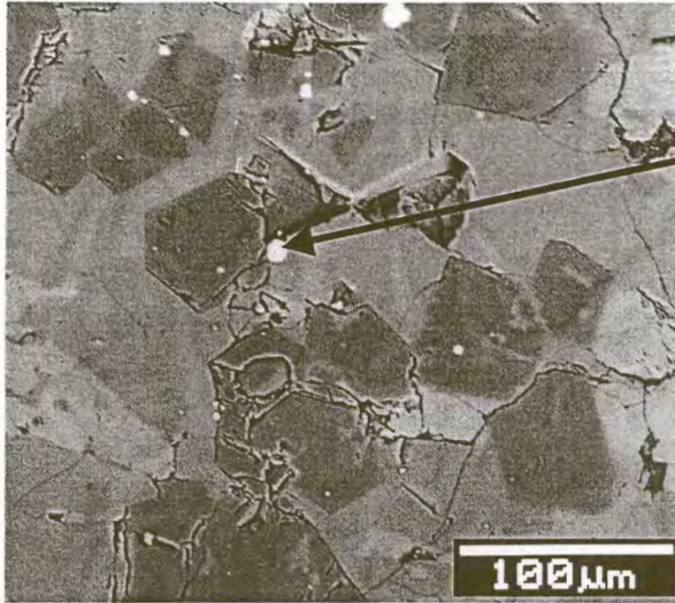
Figure 8: Back scattered electron image of vanadium droplets embedded in industrial slag sample.
