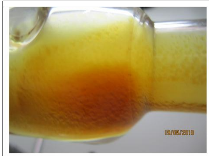
Figure 7-5 Photo of solidified wax distillate in the condenser
