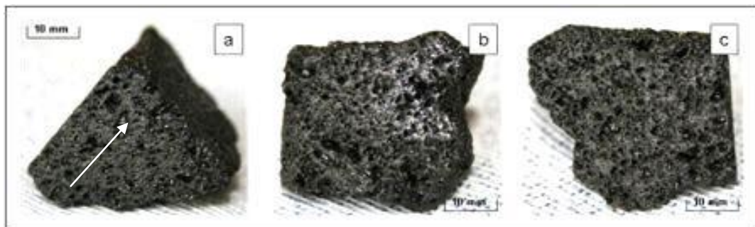
Figure 6-2 Photos (a-c) of Waxy Oil green coke (Sample 1; 1.841% ash) on an X-, Y- and Z-axis
