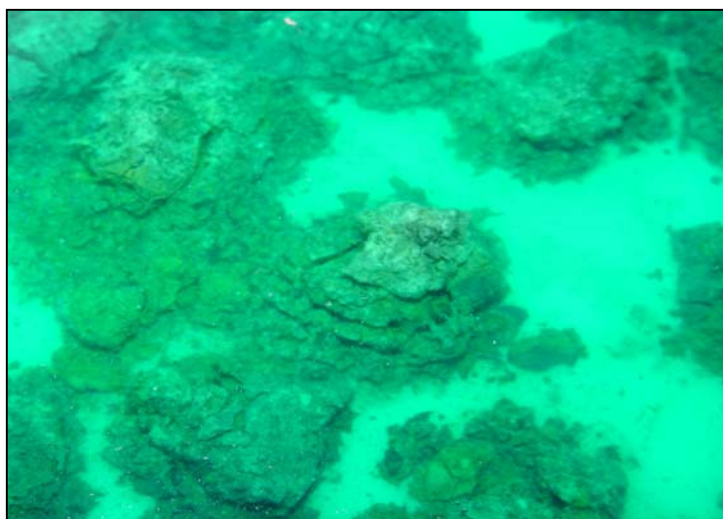
Figure 55. Visual appearance of Dutoitspan ore (initial size - 26.5 + 22.4 mm) weathered in cupric sulphate solution (0.2 M) for 24 hours.
