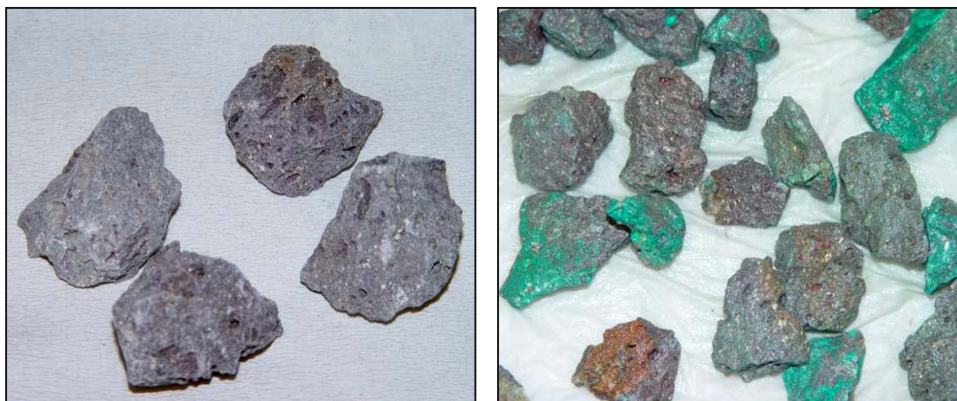
Figure 80. Venetia K8 unweathered (left) compared to the weathered product (right). Weathering was done in a 0.05 M cupric sulphate solution for 6 days.
