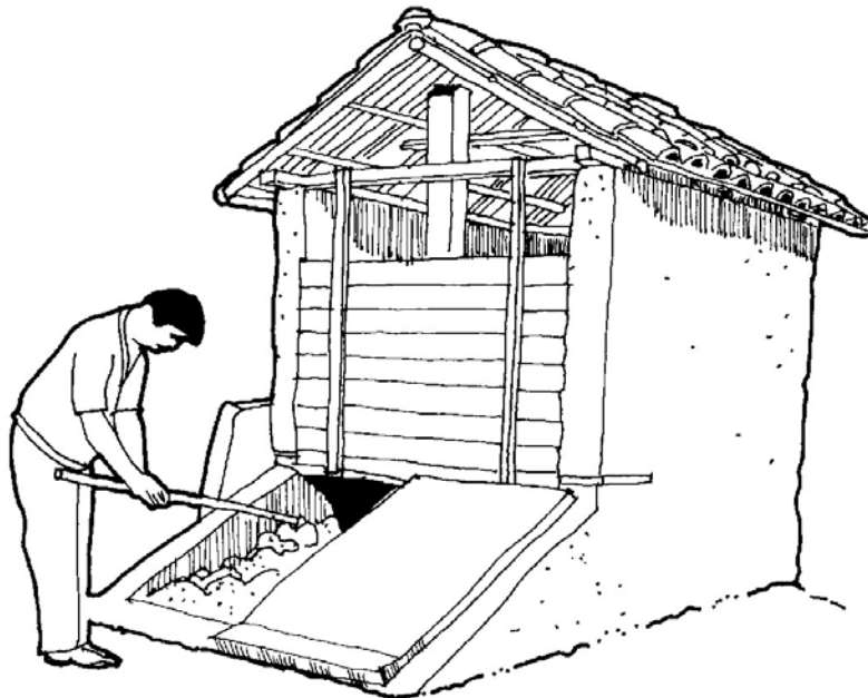
Figure 2.8: A solar-heated dehydrating toilet in Ecuador (Esrey et al 1998)
