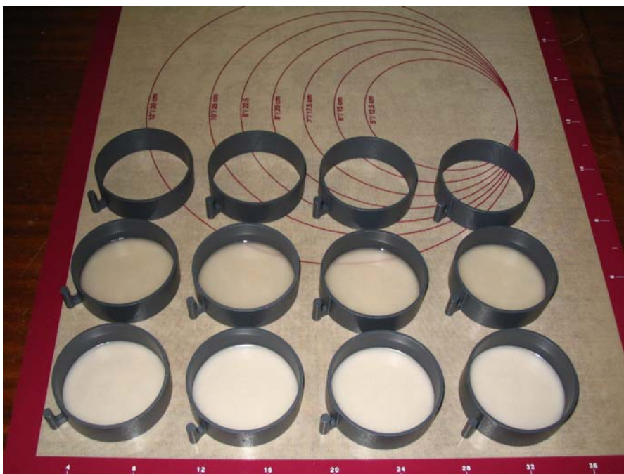
Figure 4-1 Casting of film solution into metal rings.
