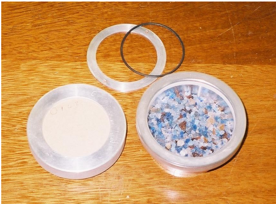
Figure 4-2 Water vapour permeability test setup.
